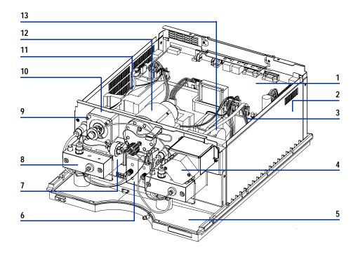
Figure 25 Nano pump main assembly
