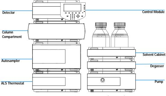
Figure 3 Recommended stack configuration (front view)
