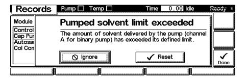
System / ErrorUse the F2-key (System Log) or F3-key (Error Log) to look for errors on the<br/>selected/ highlighted module.
