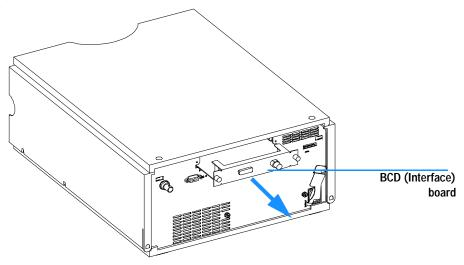
Figure 21 Exchanging the Interface Board
