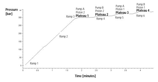
Figure 9 Typical Leak-Test Pressure Profile with IPA
