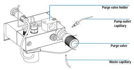
Figure 18 Exchanging the Purge Valve Frit
