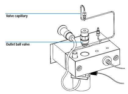
Figure 17 Exchanging the Outlet Ball Valve
