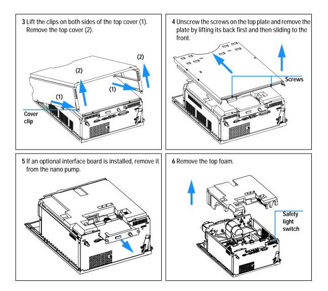
Do not connect a power plug to the nano pump module after removing the top covers.
