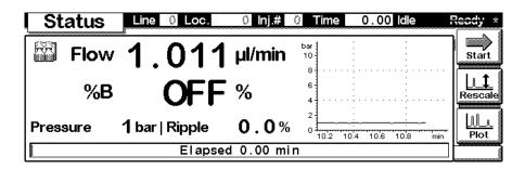
Signal plotPress F6-key (Plot) to enter the plot screen (available also from all other<br/>views). Here you can observe online signal(s). If more than one signal is<br/>configured, use the 1-2-3 numeric keys to switch between the signals.
