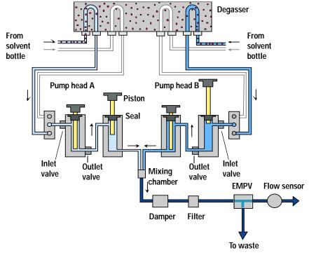
Figure 38 The Hydraulic Path
