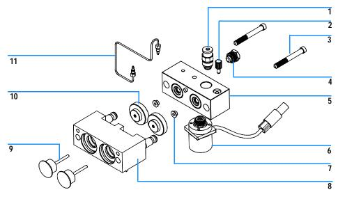
Figure 28 Pump-Head Assembly
