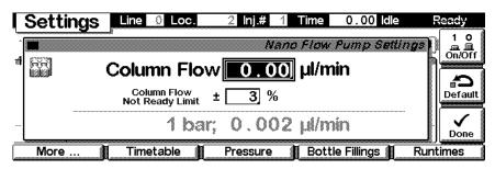
Use the **m**-key for the context sensitive menu. **Reset** will load the pump default parameters. The **Status** command pulls up the module specific setup screen.
