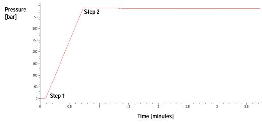
Figure 8 Typical Pressure-Test Pressure Profile with IPA
