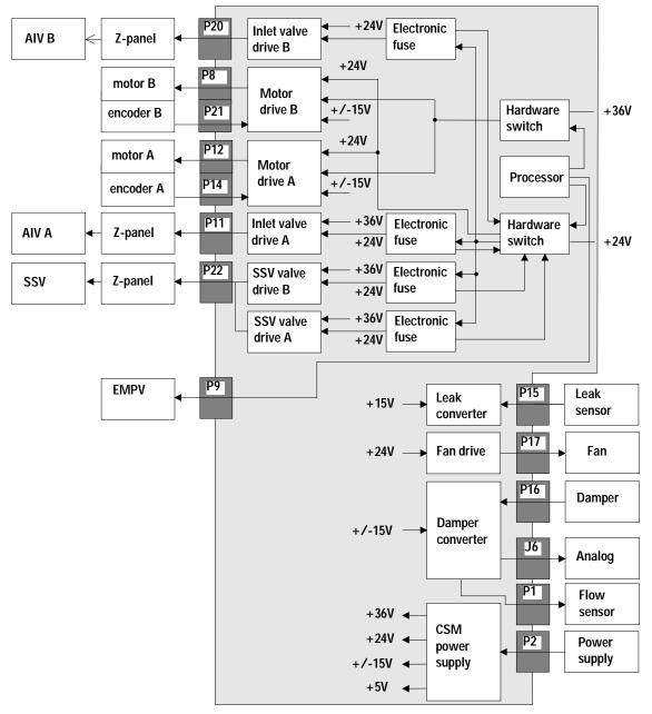
Figure 43 Interconnection Diagram NPM Board
