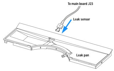
Figure 24 Exchanging the Leak Sensor
