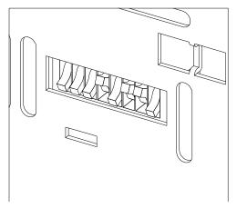
Figure 48 8-bit Configuration Switch
