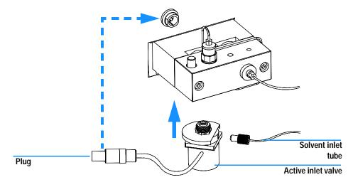
Figure 15 Exchanging the Active Inlet Valve
