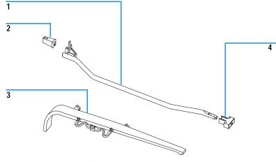
Figure 31 Power and Status Light Pipes
