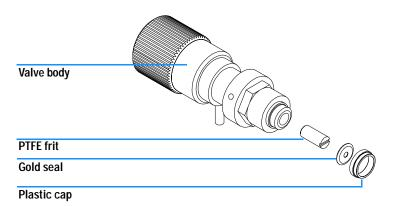
Figure 19 Purge Valve Parts
