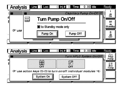
**Settings** With the **F1**-key (**Settings**) you open a pull-down menu where you can select the capillary pump module with the help of the **selection** or **alphanumeric** keys.
