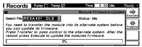
Use the **Esc**-key to receive **Views** on the **F5**-key. Choose **System** from the pull-down menu. Use the **F3**-key (**Records**) to select the **Generic** module. In this screen the resident firmware revision is shown.
