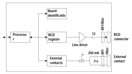
Figure 46 Block Diagram BCD Board
