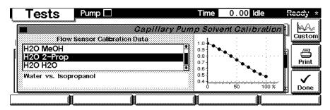
Press **Enter** once you have selected/highlighted a calibration curve to edit the individual data points of this curve. Editing the name of the curve and acknowledging the changes with **F6** (**Done**) saves the new data curve with its new name. It is possible to store one individually created calibration curve with each method. Load/Save a calibration curve from/to the PCMCIA-Card by pressing **F8** (**PC-Card**).
