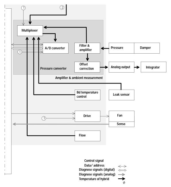
Figure 42 Block Diagram Pump Controller Board
