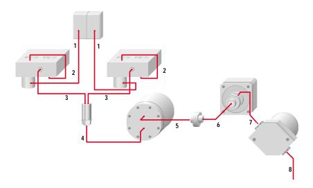
Figure 6 Flow connection of the capillary pump
