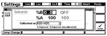
Select **Channel Selection** to choose one of the A-channels (1 or 2) and one of the B-channels (1 or 2) as the sources for solvent delivery. Changes must be activated with **F6** (**Done**).
