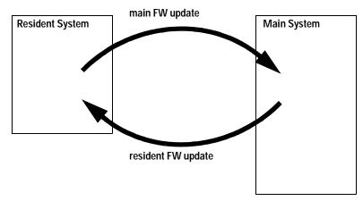
Figure 44 Firmware Update Mechanism
